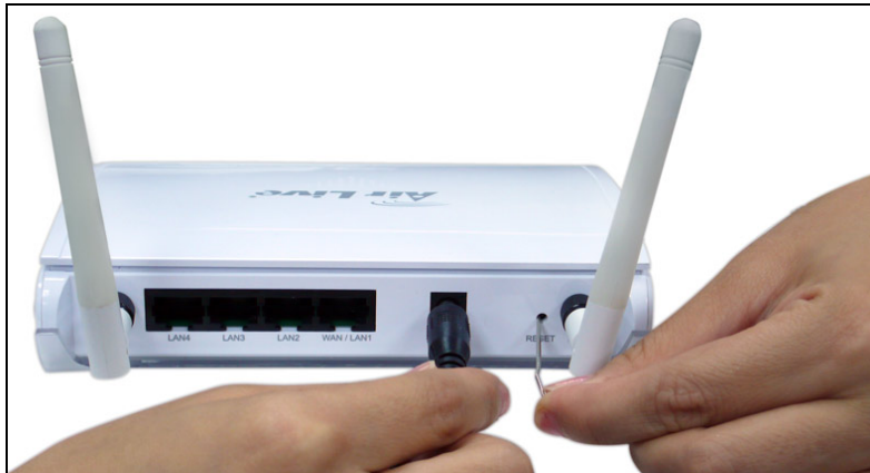
Fig 1-2 : Press and hold the reset button while plugging in the power.
